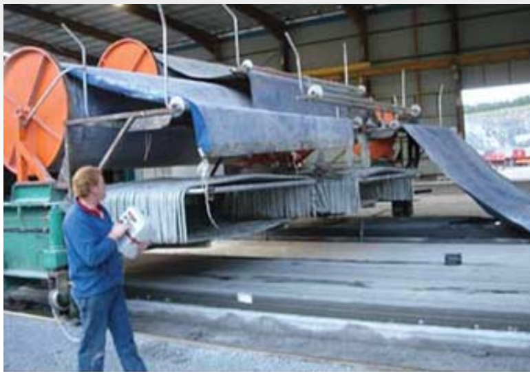
Tarping process to prepare for vapor curing of hollow-core products
